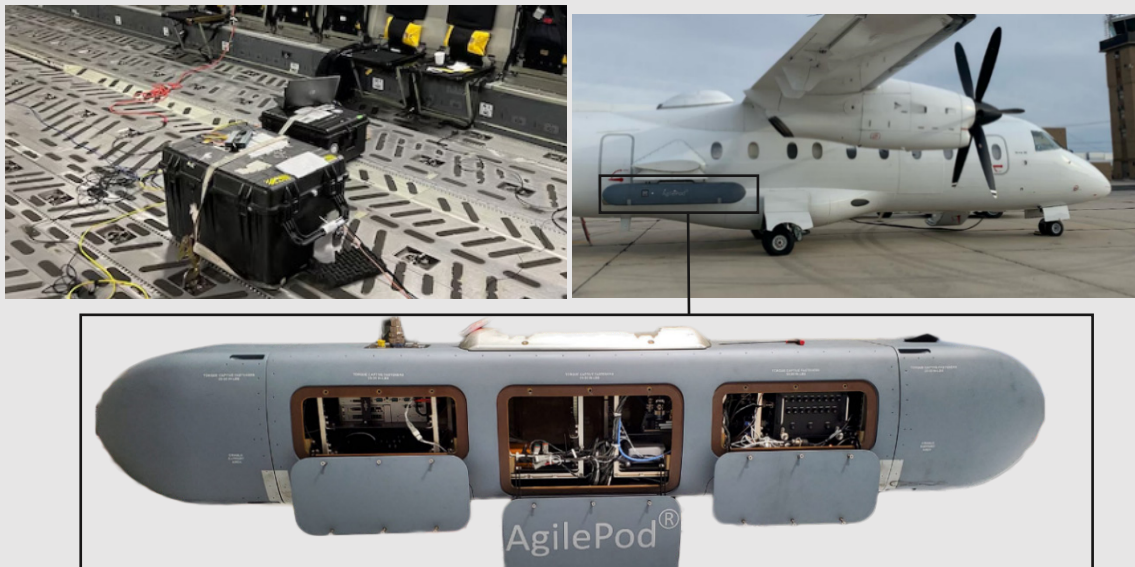
Figure 3.5: (Top Left) MagNav equipment loaded onto a DOD Aircraft prior to its first real-time demonstration. 134 (Top Right) MagNav sensors loaded in AgilePod on a DoD Aircraft prior to real-time flight test. (Bottom) Close up of the AgilePod. 135
