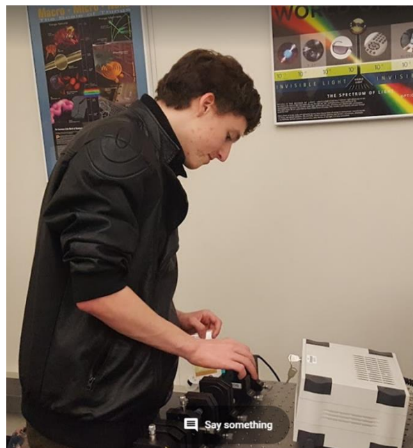
Fig. 10 is a photograph of Stefan setting up the Nd:YAG laser system. The system is not yet activated, or he would be wearing his laser safety glasses.
